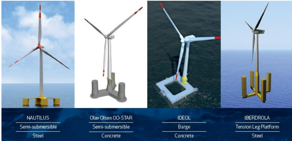
Figure 1 Offshore wind floating platform concepts considered in LIFES50+
