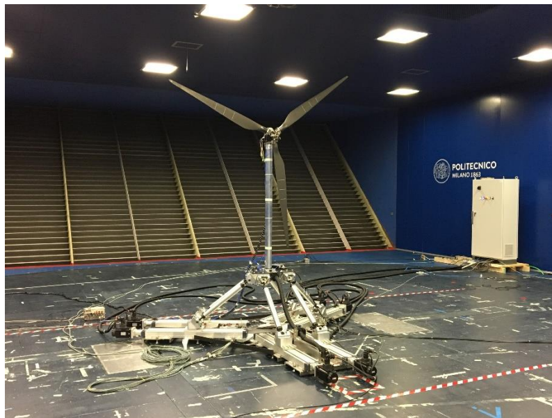
Figure 1 6-DoF robot HexaFloat coupled with 1/75 DTU 10 MW wind turbine scale model. Politecnico di Milano Atmospheric Boundary Layer.
