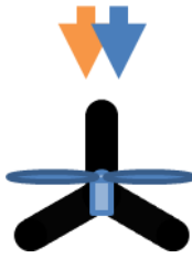
Figure 4.17: Cases of analysis to investigate platform dynamics for different environmental impact directions. LIFES50+ OO-Star Wind Floater Semi 10MW
