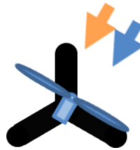
Figure 4.17: Cases of analysis to investigate platform dynamics for different environmental impact directions. LIFES50+ OO-Star Wind Floater Semi 10MW
