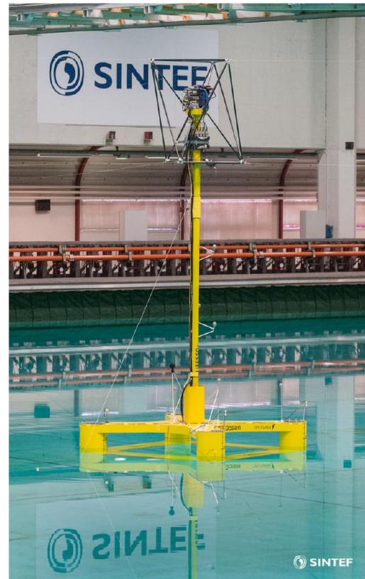
Figure 33: NAUTILUS-DTU10 scaled model in the wave basin at SINTEF [30].
