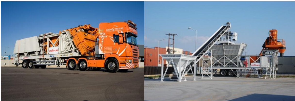
Figure 19: Left: Mobile batch plant during transportation [12]; Right: Examples of quick assembly plant modules [12].
