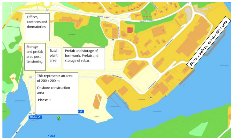
Figure 15: Proposed layout for fabrication and assembly (Farsund, concrete).
