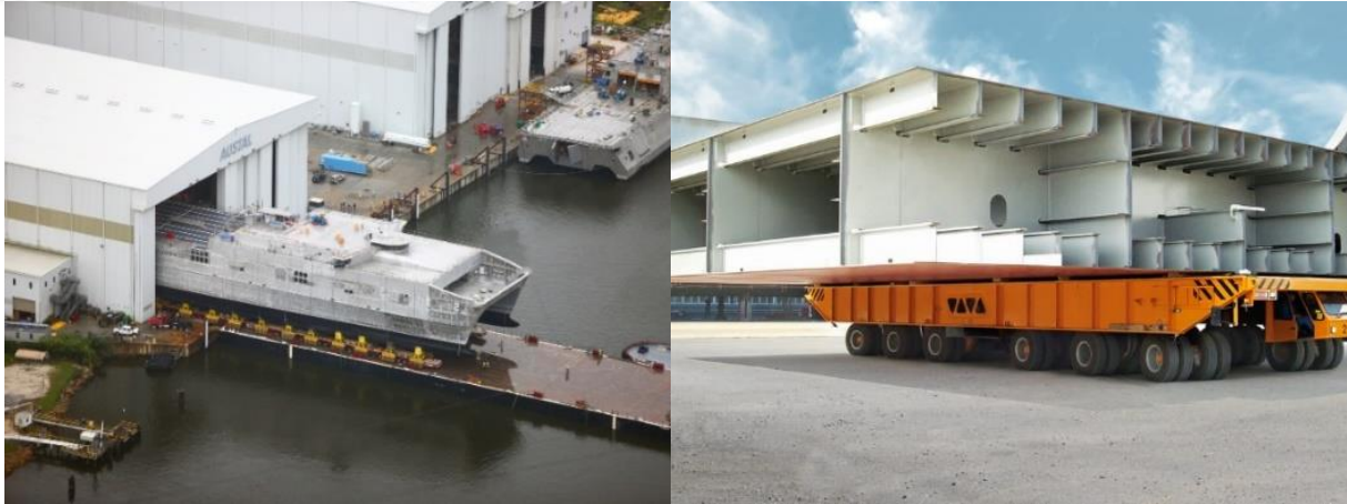
Figure 21: Left: Transfers of vessel onto barge using SPMT [15]; Right: Shipyard transporters by KAMAG with payloads of up to 1300 tonnes [16].
